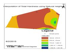
This spatially interpolated water quality map will be helpful in determining the contamination range troughout the boundary of the tank.
