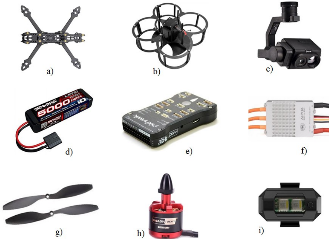
Fig 3: a) Drone Frame b) Release Mechanism c) Thermal Image Camera d) Li-Po Battery e) Flight Controller f) ESC g) Propeller h) BLDC Motor i) LED Lights
