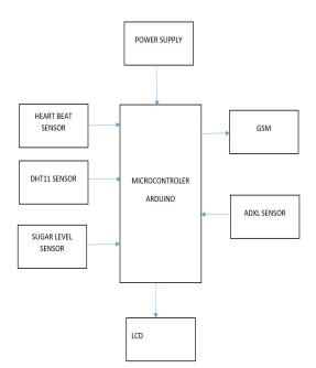
Equipped with advanced processing capabilities, the microcontroller manages incoming sensor data, detects anomalies, and triggers appropriate responses or alerts as necessary. This centralized control enhances the system's efficiency and responsiveness, facilitating real-time monitoring and proactive management of maternal and fetal health
