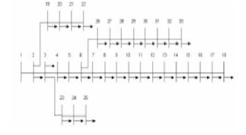
Fig 2 Online diagram of IEEE 33 – bus radial district 6.6.1 PROGRAMING DATA
