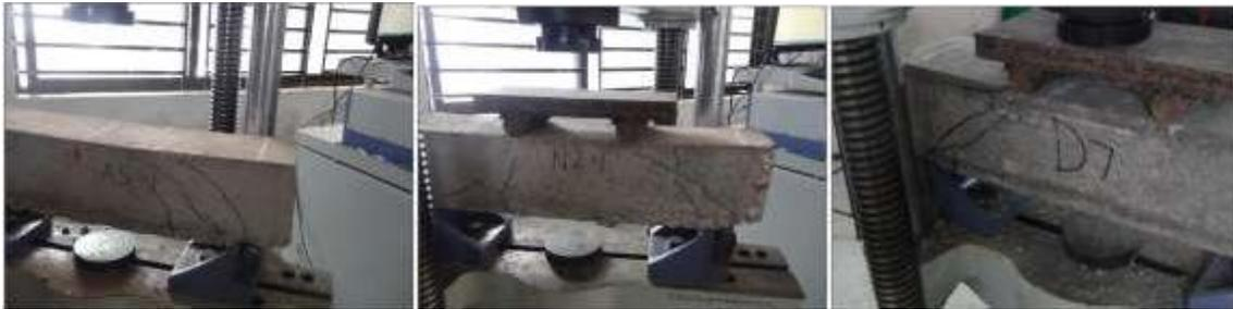
Fig. No. 6: crack pattern for B1, B2, B3 beams with shear reinforcement
