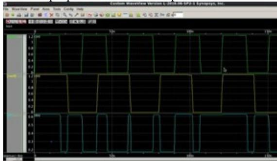
Fig 5: Output Waveform of proposed 3T XNOR Gate
