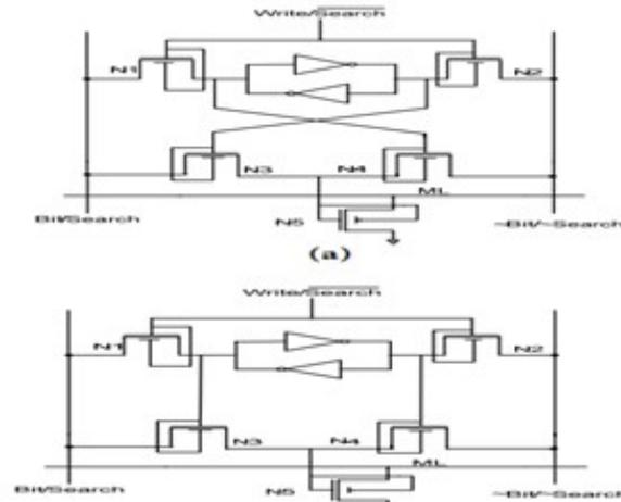
Figure 9. Typical XNOR-XOR Cell. (a) XOR type. (b) XNOR type.
