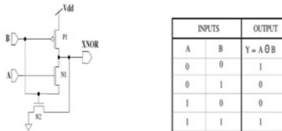
Fig 2: Existing 3T XNOR Gate Table1: Truth table of XNOR logic gate
