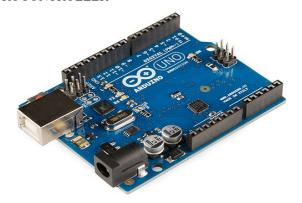
A microcontroller board based on the ATmega328 IC is called the Arduino Uno R3. There were 6 analog inputs, a 16 MHz crystal oscillator, a USB port, 14 digital input/output pins (six of which may be utilized as PWM outputs), a power button for resetting, an ICSP header, and a jack. Everything required to support the microcontroller is included; all that's left to do is power it with a battery or an AC-to-DC adapter or connect it to a computer via a USB cable.
