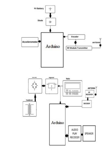
5. SYSTEM REQUIREMENTS HARDWARE DESCRIPTION 5.1Power Supply The 12V advanced step-down transformer is powered by an AC source. The 12V AC transformer is rectified by means of a diode connection. A capacitor separates the 12V DC diode bridge yield. 5.2 LCD Display
