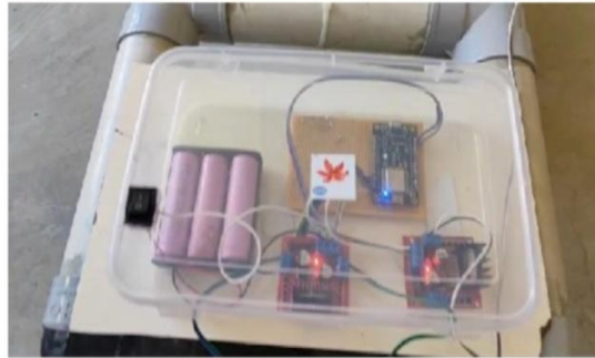
Fig 4. The thruster module with the motor driver CONCLUSION
