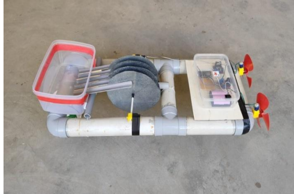
Fig 3. Top view of the disc-type oil skimmer in hardware setup
