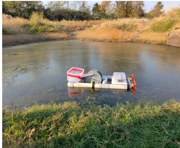
Fig 2. Real-time implementation of an IoT integrated Double Disc type oil skimmer module
