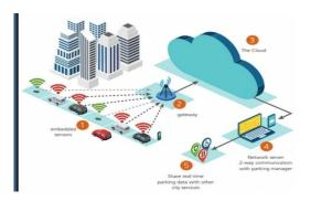
Our proposed solution aims to harness IoT sensors strategically deployed within parking slots to detect the presence of vehicles. These sensors will be equipped to wirelessly transmit data to a centralized system for efficient processing and analysis.
