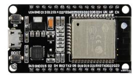
It combines the power of the ESP32 chip with the convenience of the NodeMCU platform, making it ideal for Internet of Things (IoT) projects. With built-in Wi-Fi and Bluetooth capabilities, digital and analog input/output pins, and support for various programming languages including Arduino and Micro Python, the NodeMCU ESP32 is widely used for prototyping and building IoT devices in applications such as home automation, remote monitoring, and industrial automation.
