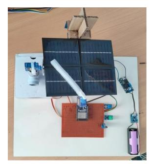
mplementing a self-optimizing dual-axis solar panel system using IoT technology involves integrating various hardware components for sun tracking, panel angle adjustments, temperature monitoring, cleaning mechanisms, and remote monitoring. Below is a hardware implementation overview:
