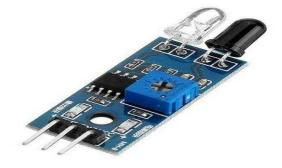
The LM393 comparator-based infrared sensor is commonly used in applications such as proximity sensing, object detection, and line following in robotics. The comparator helps in comparing the voltage levels from the infrared sensor and providing a digital output based on the comparison.
