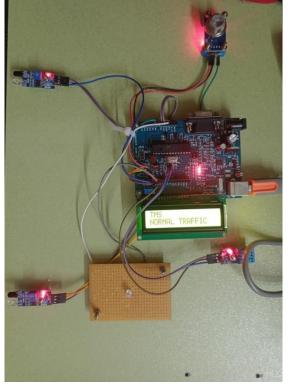
• The temperature sensor is used to measure the heat index, temperature and humidity present in the environment.
