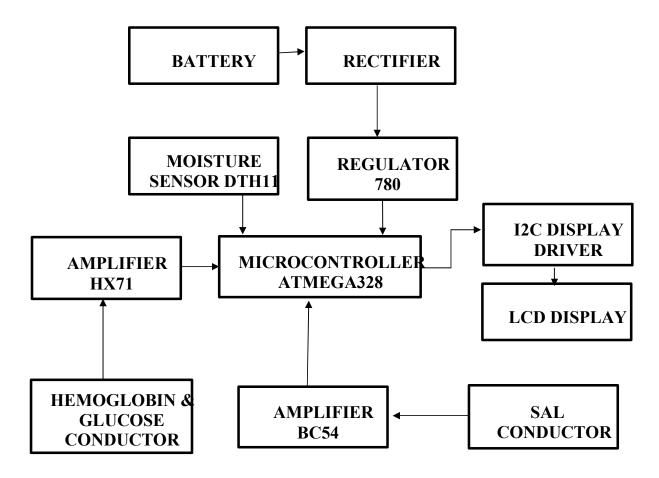
Figure 1. Block diagram of Micro Fluidic Hemoanalyzer
