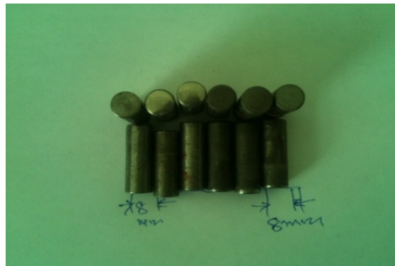
Figure-1 Macrographs of pins (specimen) prepared for coatings on end faces
