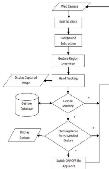
Figure 1. Proposed block diagram of hand gesture recognition.
