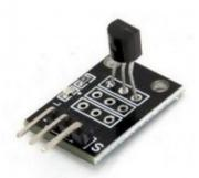
The device used here is DS18B20. It's a digital thermometer which has an alarm functions, upper and lower trigger points. They are non-volatile. The temperature measured is of range 9-12 bit Celsius. They are accurate and easy to take measurements. Their outputs are connected to GPIO22 Pico board. 3. Pulse Sensor
