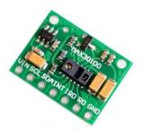
The volume of the blood changes according to the heart pumping and this can be detected by using pulse sensor. The heart rate can be measured by four methods includes ECG, Photoelectric pulse wave, blood pressure readings and phonocardiography. Pulse sensor uses photoelectric technique. The techniques used for
