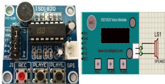
Fig 7 Voice Module device with Pin Configuration
