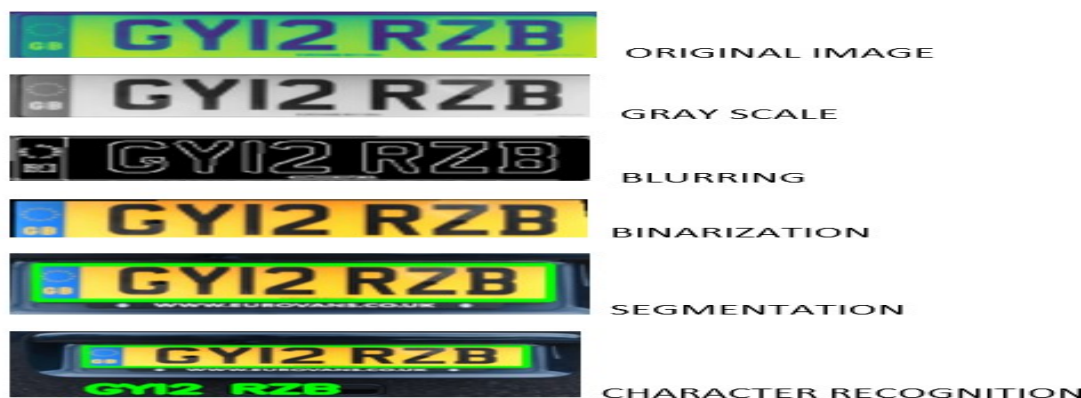
Fig 1. Process of extraction from a number plate
