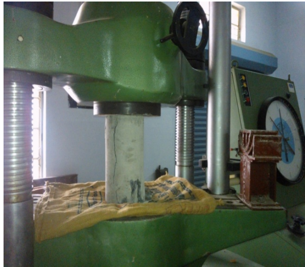
Fig. 6. Behavior of cylinder under compression
