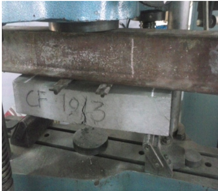
Fig. 8. Behavior of prism under flexure
