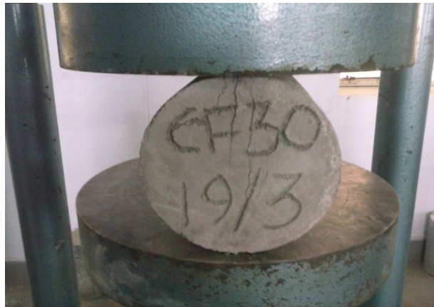
Fig. 4. Behavior of cylinder under split tension
