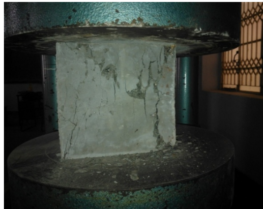
Fig. 2. Behavior of cube under compression
