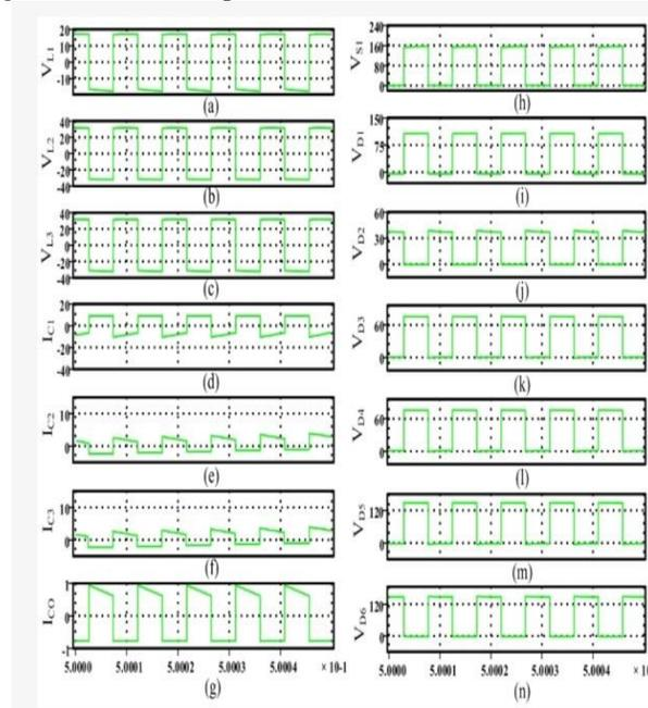
Figure 14. Simulation results: (a) first inductor voltage, (b) second inductor voltage, (c) third inductor voltage, (d) first capacitor current, (e) second capacitor current, (f) third capacitor current, (g) output capacitor current, (h) switch voltage, (i) first diode voltage, (j) second diode voltage, (k) third diode voltage, (l) fourth diode voltage, (m) fifth diode voltage, (n) sixth diode voltage.
