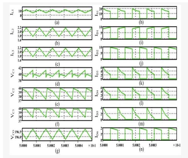
Figure 3. Simulation results: (a) first inductor current, (b) second inductor current, (c) third inductor current, (d) first capacitor voltage, (e) second capacitor voltage, (f) third capacitor voltage, (g) output capacitor voltage, (h)
