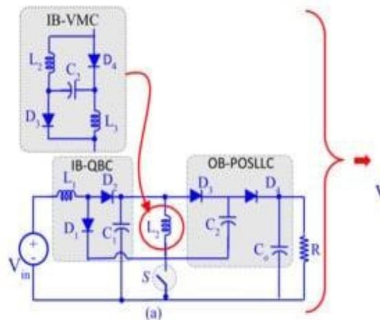
Figure 2. (a) The composition of the proposed converter,
