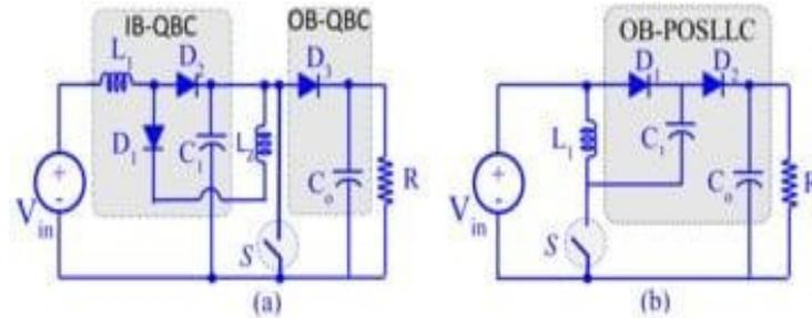
Figure 1. (a) Cascaded boost converter, Figure 1. (b) positive output super lift Luoconverter, Figure 1. (c) modified form of the boost converter by a voltage multiplier cell.
