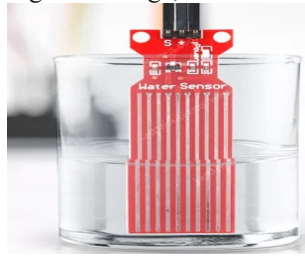
Fig. 2 Water Level Sensor
