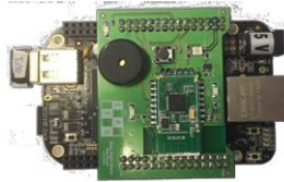
Gateway: shield placement on the Beagle Bone Black
