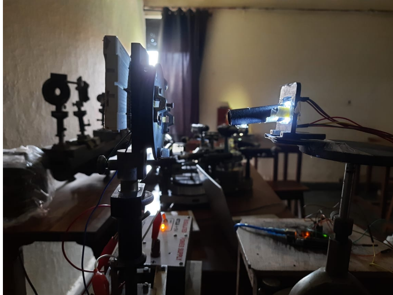
Figure 7: Experimental setup for determining the wavelength of light sources
