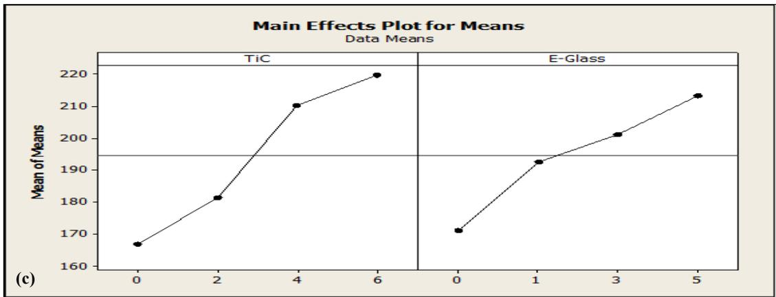
Figure 1 Effect of individual parameters on ultimate tensile strength value of Al 2024 / TiC / E-Glass (a) TiC, (b) E-Glass, and (c) graph obtained from mini stab statistical tool.
