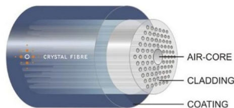
Figure 4. Cross-section of a photonic band-gap fibre.
