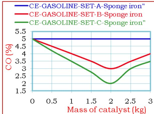
Figure 8 Variation of CO emissions at full load operation of the base engine with the mass of SPI catalyst under various working sets of catalytic converter
