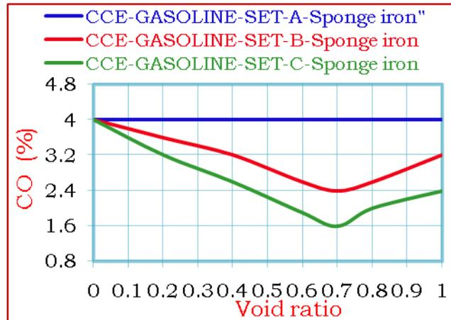
Figure 6 Variation of CO emissions at full load operation of CCE using base fuel with void ratio under various working sets of catalytic converter with SPI catalyst
