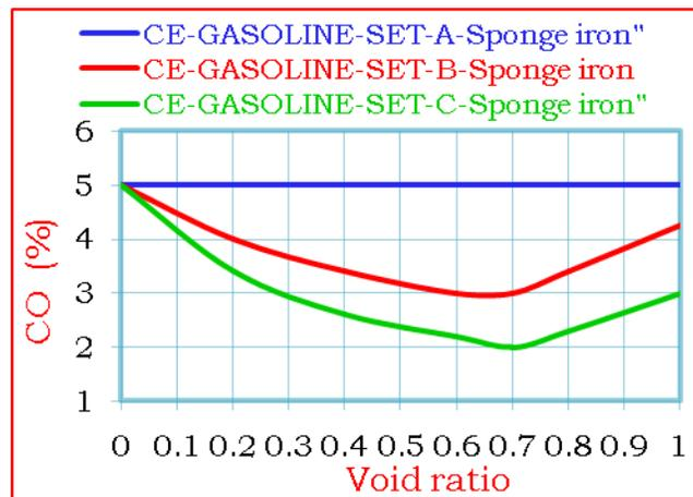
Figure 4 Variation of CO emissions at full load operation of the base engine with void ratio under working sets of catalytic converter with SPI catalyst
