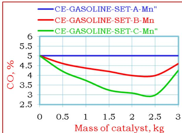
Figure 9 Variation of CO emissions at full load operation of the base engine with the mass of Mn ore catalyst under various working sets of catalytic converter
