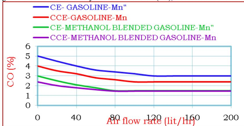
Figure 13 Variation of CO emissions with air flow rate in the catalytic converter using test fuels and Mn ore catalyst for base engine and catalytic coated engine
