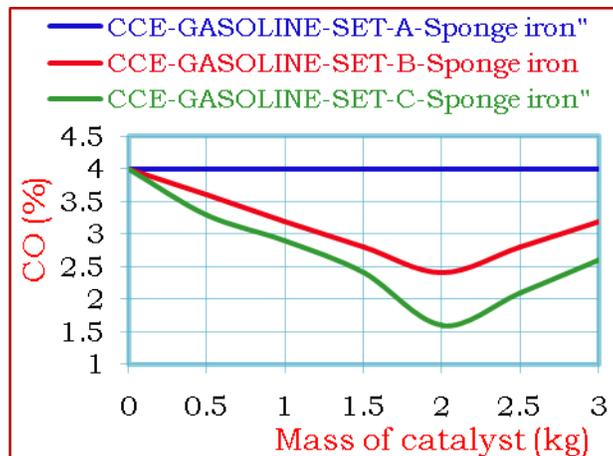
Figure 10 Variation of CO emissions at full load operation of CCE using base fuel with the mass of SPI catalyst working under various sets of catalytic converter
