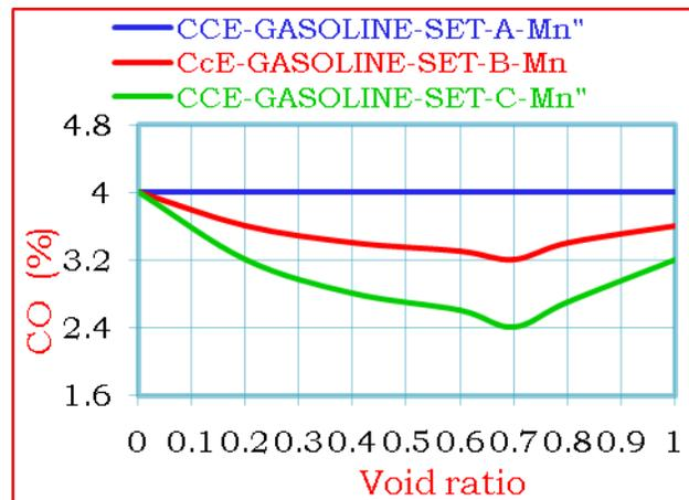
Figure 7 Variation of CO emissions at full load operation of CCE using base fuel with void ratio under working sets of catalytic converter with Mn ore catalyst
