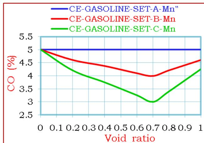
Figure 5 Variation of CO emissions at full load operation of the base engine with void ratio under working sets
