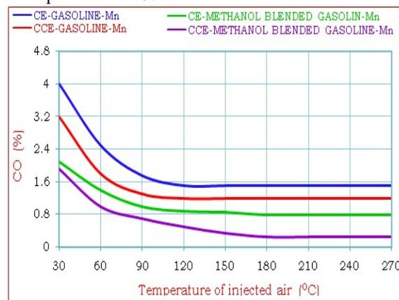
Figure 15 Variation of CO emissions with the temperature of air injected in to the catalytic converter for the base engine and CCE using test fuels and Mn ore catalyst
