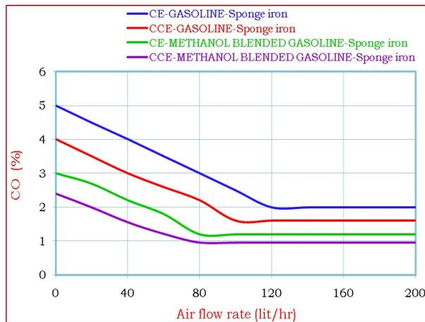
Figure 12 Variation of CO emissions with air flow rate in the catalytic converter using test fuels and SPI catalyst for the base engine and catalytic coated engine
