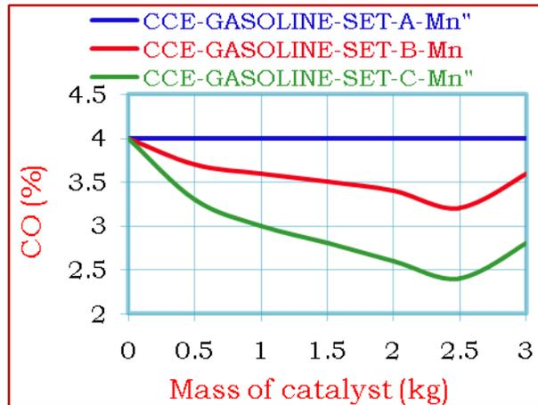
Figure 11 Variation of CO emissions at full load operation of CCE using base fuel with the mass of Mn ore working under various sets of catalytic converter
