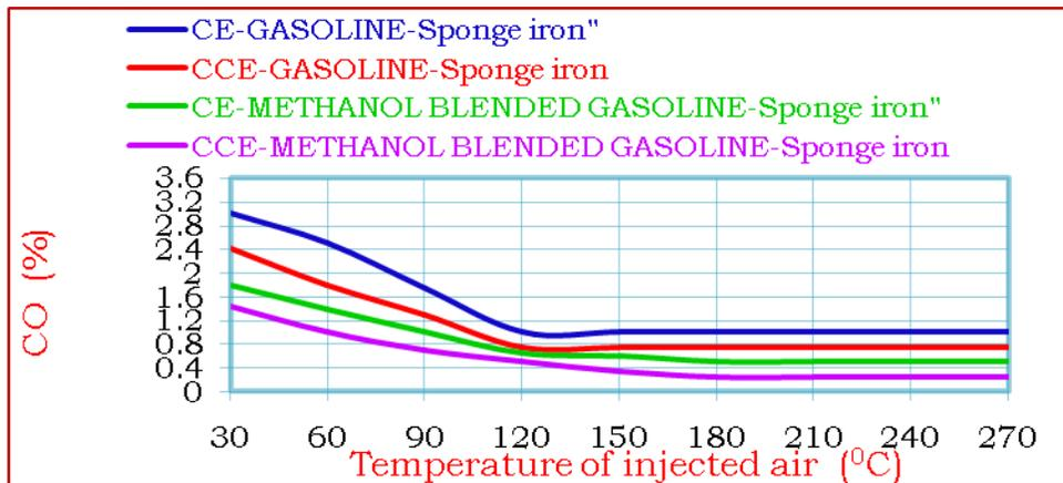
Figure 14 Variation of CO emissions with the temperature of air injected in to the catalytic converter for the base engine and CCE using test fuels and SPI catalyst
