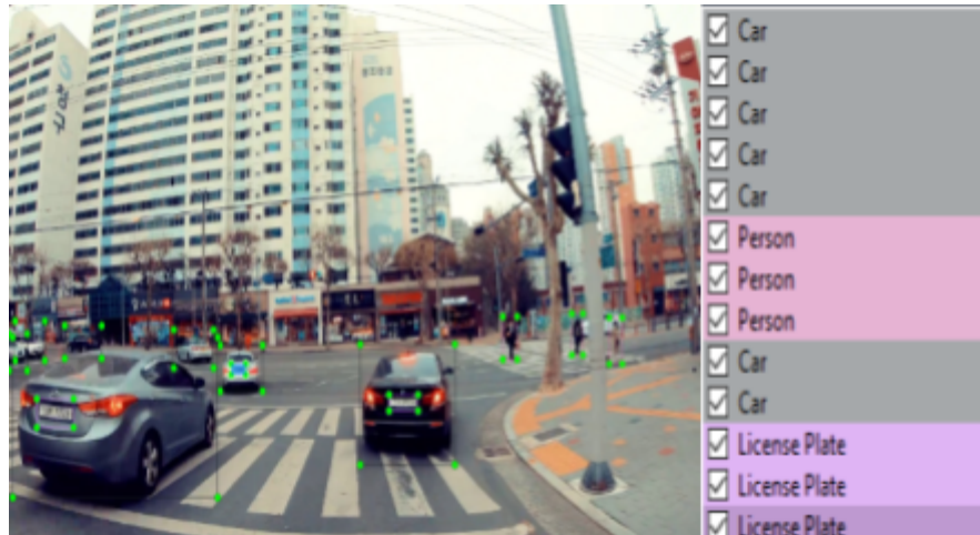
Figure 3. Annotation process. (a) The top left green point represents the starting point of every bounding box annotation. (b) Total 13 object instances labelled, and three type categories have occurred
