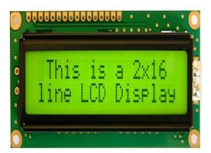
A **liquid crystal display** (**LCD**) is a thin, flat electronic visual display that uses the light modulating properties of liquid crystals (LCs). LCs do not emit light directly.
