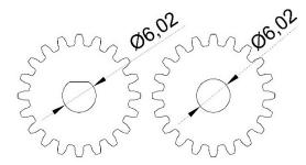
The gears in a transmission are analogous to the wheels in a crossed, belt pulley system. An advantage of gears is that the teeth of a gear prevent slippage. When two gears mesh, if one gear is bigger than the other, a mechanical advantage is produced, with the rotational speeds, and the torques, of the two gears differing in proportion to their diameters.
