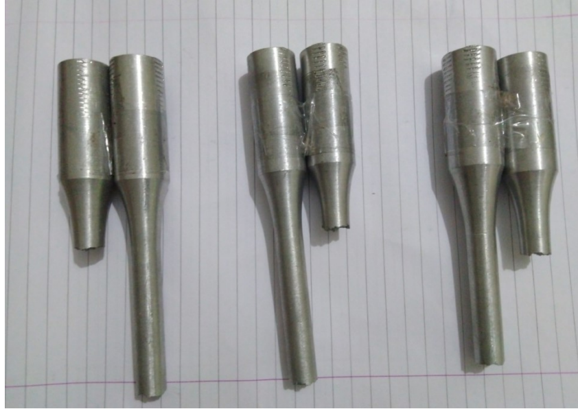
Fig no. 2 Tensile strength samples
