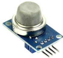
Figure 3.4: Pictorial diagram of Gas Sensor
