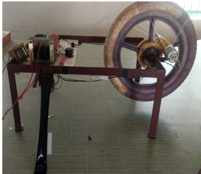
Fig 5- Two wheeler is off condition (key and wheel )
