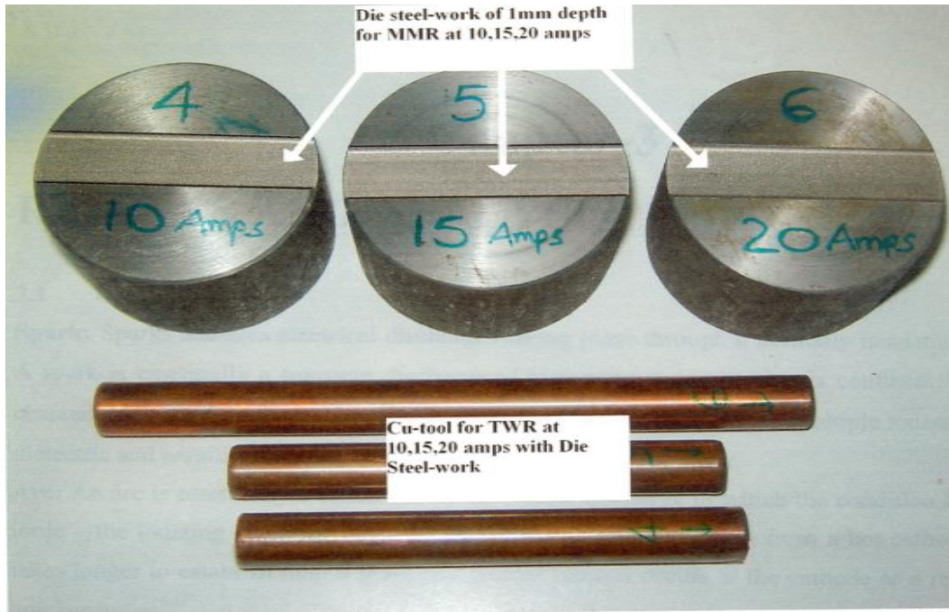
Photo5-Copper tool, Die steel work piece (above)
