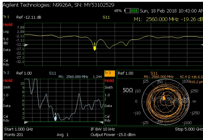
Figure 11. Measured value of S11 and VSWR
