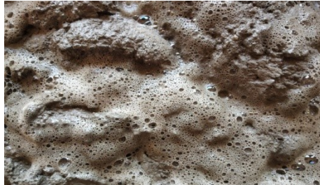
Figure 3. Preparation of the mix using pre-foaming method
