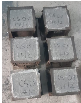
Figure2. Casting of concrete cube
