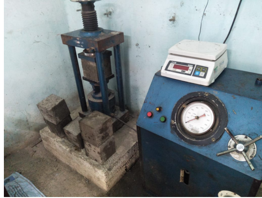
Figure 3. Compressive strength test of concrete
