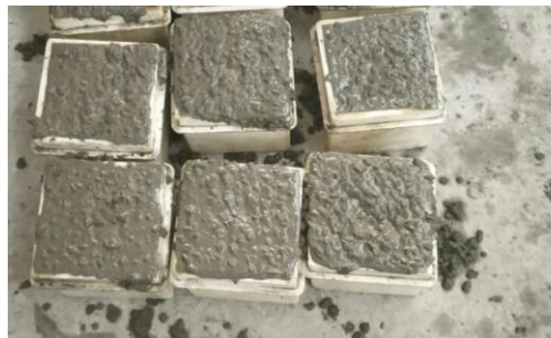
Figure 3. Casting of concrete
