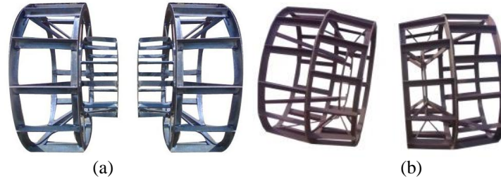
Figure 1. (a) Half cage (b) Full cage ( image courtesy by the Trichy agro Industries)
