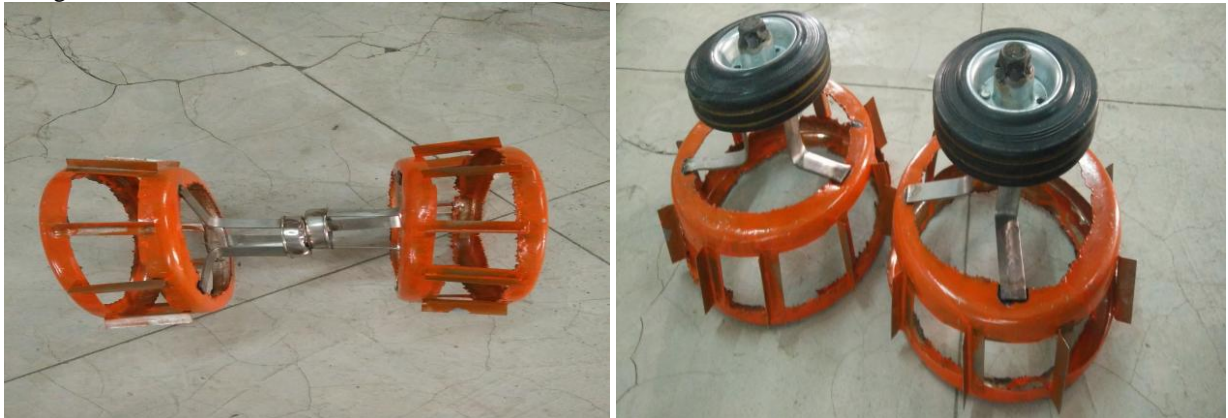
Figure 7. Fabrication of cage wheel
