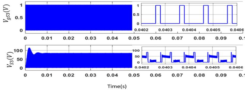
Figure 14: (a) Gate pulse ( $V_{gS3}$ ), (b) Voltage across switch ( $V_{S3}$ )
