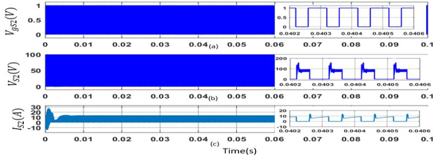
Figure 13: (a) Gate pulse ( $V_{gS2}$ ), (b) Voltage across switch ( $V_{S2}$ ), and (c) Current through switch ( $I_{S2}$ )
