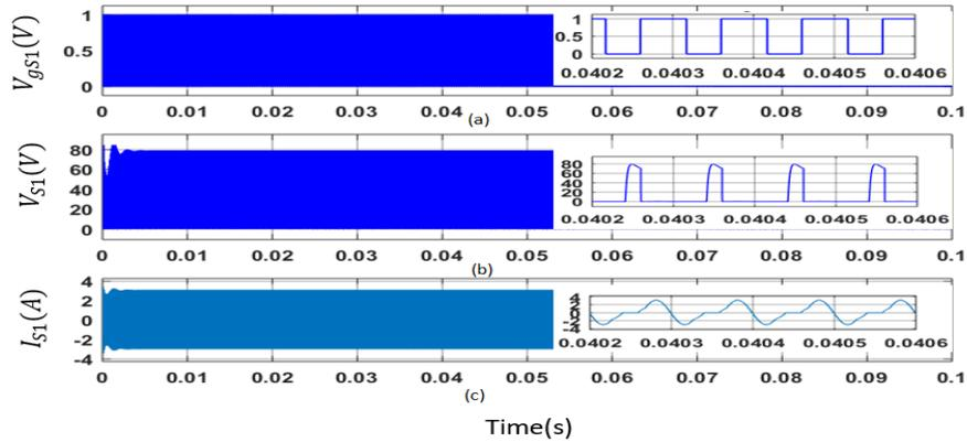
Figure 9. (a) Gate pulse ( $V_{gS1}$ ), (b) Voltage across switch ( $V_{S1}$ ), and (c) Current through switch ( $I_{S1}$ )
