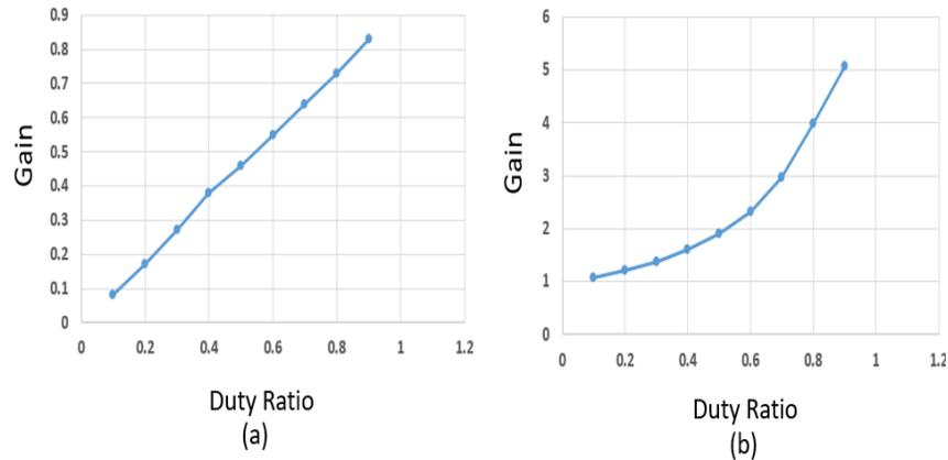
Figure 16: (a) Gain vs Duty ratio for Buck mode (b) Gain vs Duty ratio for Boost mode
