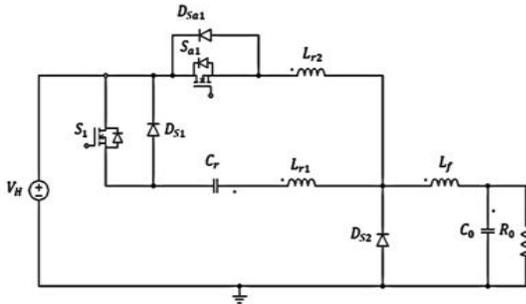
Figure.2.The configuration of the proposed BDC in Buck mode
