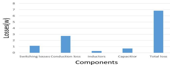
Figure 17: Power Loss Distribution Of Components
