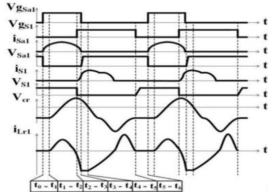
Figure.3. Theoretical Waveforms in Buck mode
