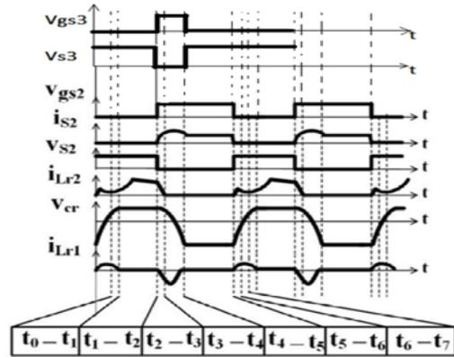
Figure.5. The configuration of the proposed BDC in Boost mode    Figure.6. Theoretical Waveforms in Boost mode
