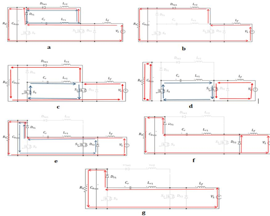
Figure.7. Modes of operation in Boost mode
