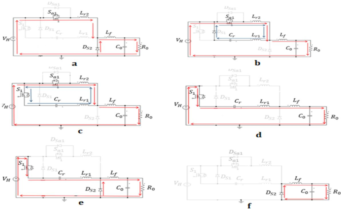
Figure.4. Modes of Operation in Buck mode
