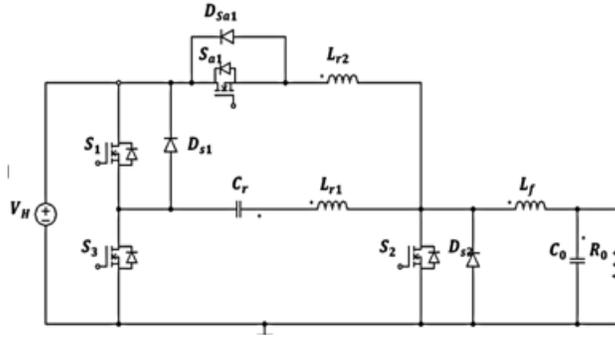
Figure.1. Soft Switched BDC with Reduced Losses
