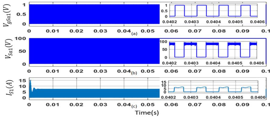
Figure 10: (a) Gate pulse ( $V_{gSa1}$ ), (b) Voltage across switch ( $V_{Sa1}$ ) and (c) Current through switch ( $I_{Sa1}$ )
