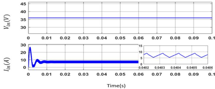
Figure 11: (a) Input Voltage ( $V_{in}$ ), (b) Input Current ( $I_{in}$ )
