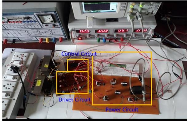
Fig 18: Top view of the experimental setup
