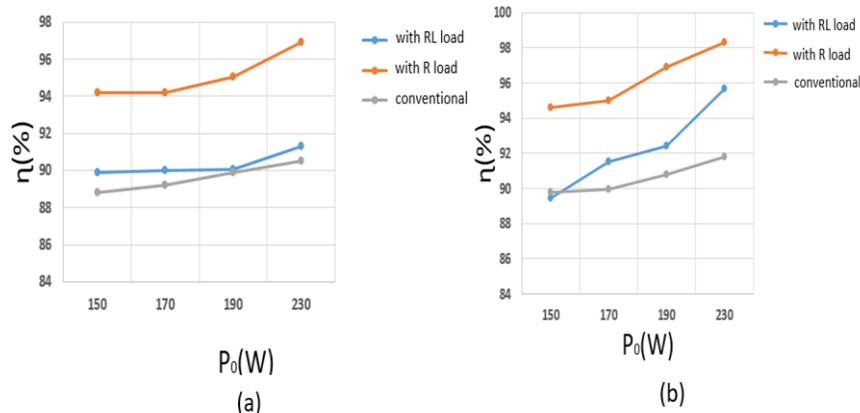
Figure 15: (a) Efficiency of the converter in Buck mode (b) Efficiency of the converter in Boost mode
