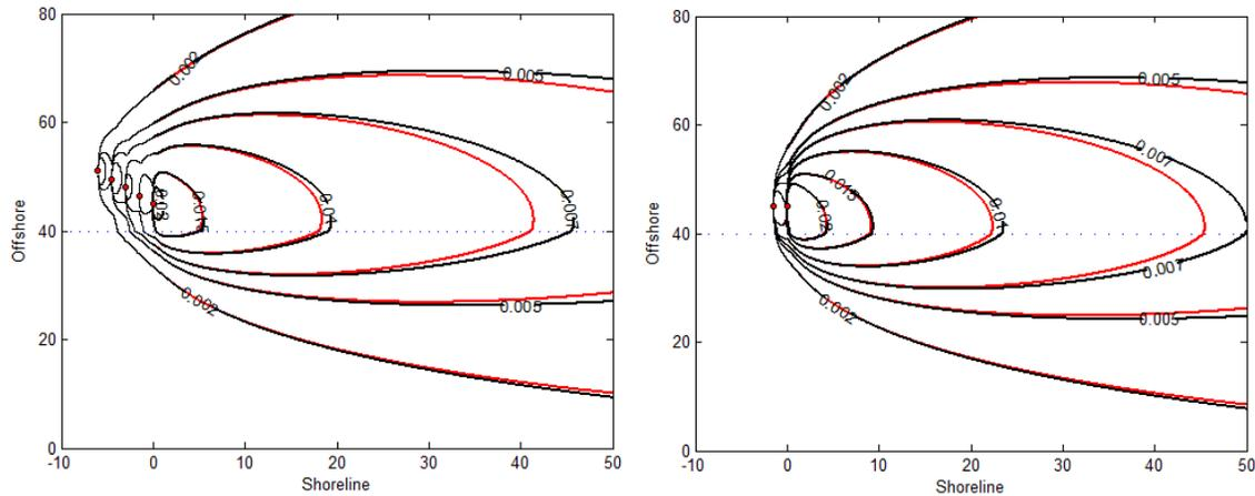
Figure 3 Contours of solutions for effluents discharge at  $\alpha = 45$  with  $\lambda = 0.2$  on a step seabed when  $\ell = 40$  and  $r = 2$  for: five points source with  $d = p = 1.5$  (left); and two points source with  $d = 1.5$ ,  $p = 0$  (right). The case of no decay  $\gamma = 0$  (black contour) and decay of  $\gamma = 0.0005$  that increases with depth  $\sigma = 1$  (red contour)
