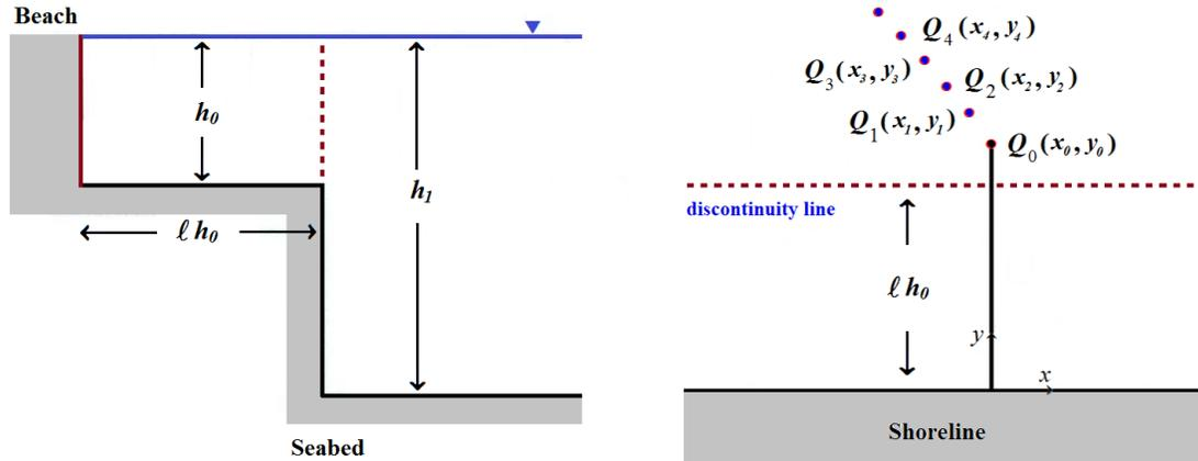
Figure 1 Cross-section depth profile of a step seabed (left); and diagram of multiple point sources representing a multiport diffuser (right)
