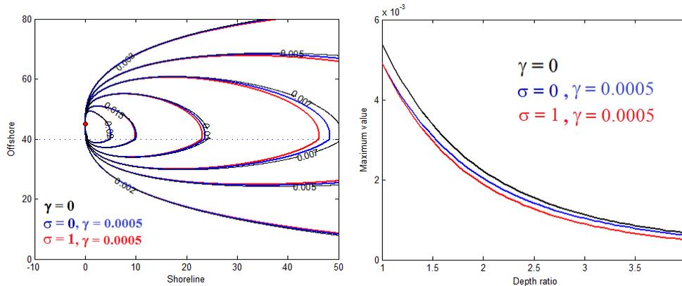
Figure 4 Contours of solutions for effluents discharge from a point source at  $\alpha = 45$  with  $\lambda = 0.2$  on a step seabed when  $\ell = 40$  and  $r = 2$  (left); and the maximum value  $C_{0m}$  of concentration at the shoreline (right). The case of no decay  $\gamma = 0$  (black contour), constant decay of  $\gamma = 0.0005$  and  $\sigma = 0$  (blue contour), and decay of  $\gamma = 0.0005$  that increases with depth  $\sigma = 1$  (red contour)
