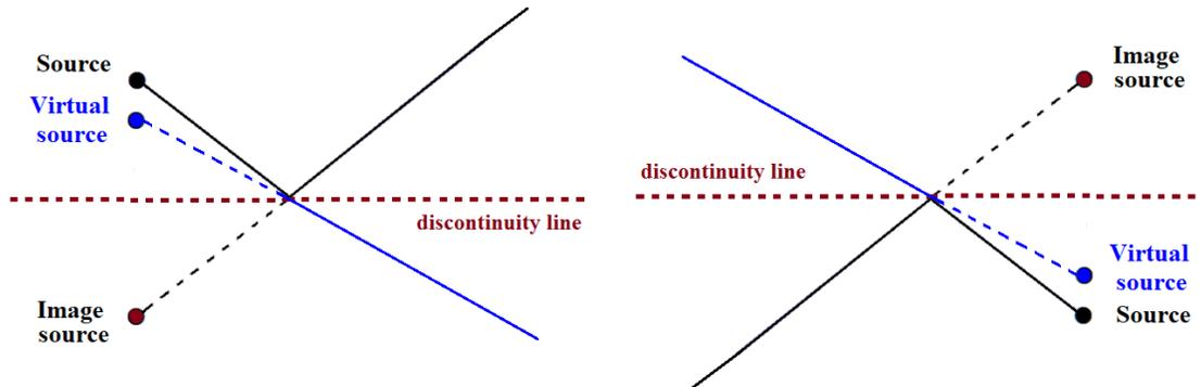
Figure 2 Diagram of the positions of the (actual) source, image source, and virtual source used in the method of image
