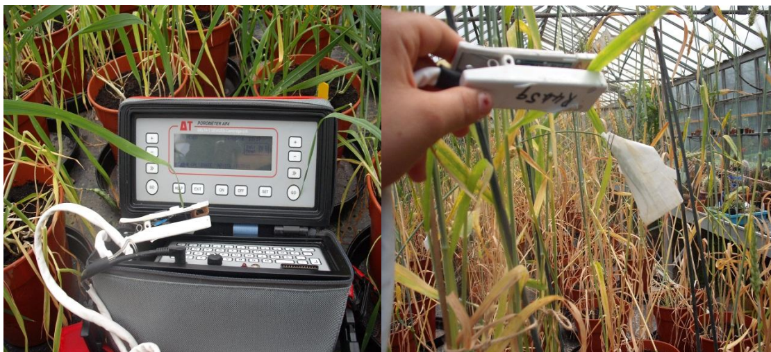
Figure (3): AP4 porometer was used for measuring the stomatal resistance
