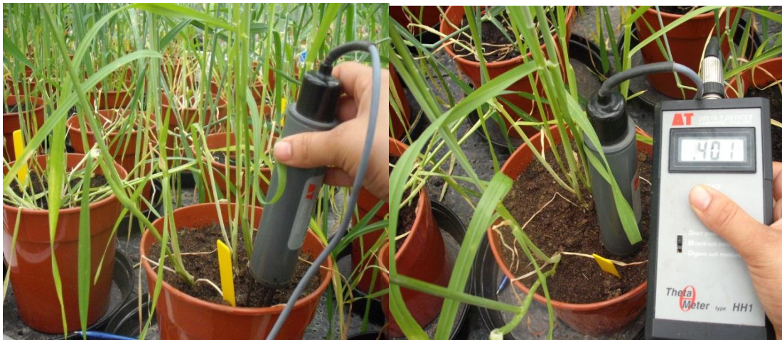
Figure (2): Theata Meter was used for measuring soil moisture
