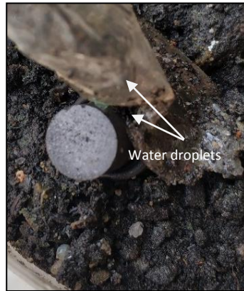
Figure 10. Water droplets forming on the surface of cathode due to the recombination of hydrogen atom with oxygen from the air
