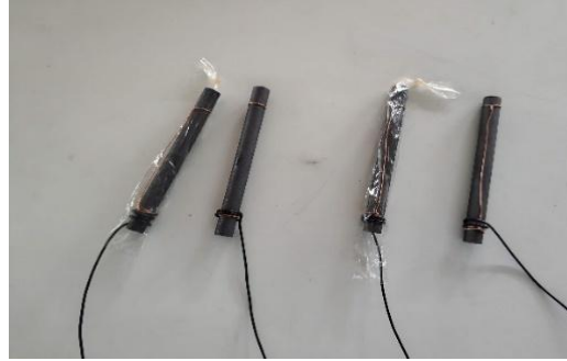
Figure 3 Preparation of graphite electrodes for the P-MFC. The cathodes are wrapped in a cellulose membrane and the anodes are without a membrane.
