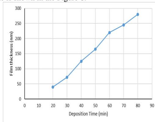
Figure 8: Thickness of the AZO films at different deposition time.
