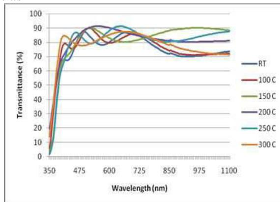
Figure 10: Optical transmittance spectra of ZnO:Al films
