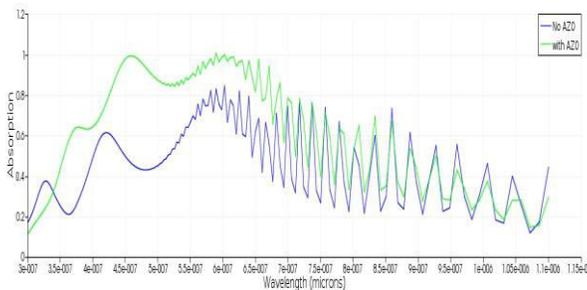
Figure 6: Effect of TCO coating on Solar cell
