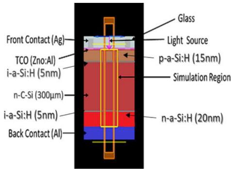
Figure 1: Simulation block diagram.
