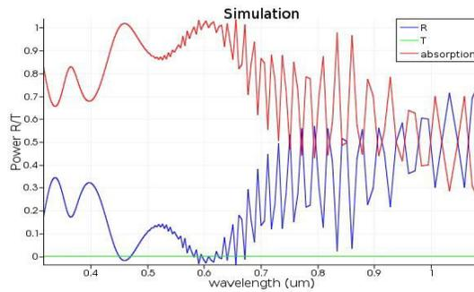
Figure 2: Simulated reflection, transmission and absorption of the C-Si Solar cell with TCO
