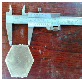
Fig.2.4 Specimen checked for dimensions
