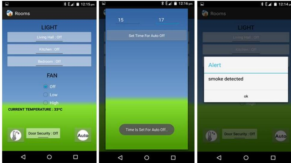
Figure 6. GUI of Android Application showing temperature, auto off time set and smoke detection alert.
