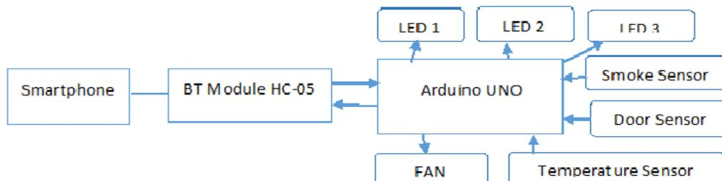
Figure 3. Block diagram of smart automation system using Bluetooth
