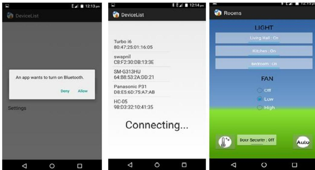
Figure.5. GUI of Android Application showing process of connecting to Bluetooth module.
