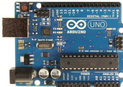
Figure 1. Arduino Uno Board
