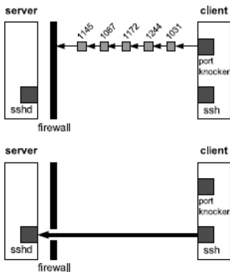
Figure 2: Port knocking example. The firewall is opened in response to a specific port sequence used for authentication.
